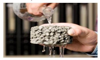
Figure 1 Pervious Concrete
