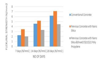
Figure 10 Results for Flexural Strength
