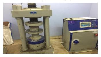
Figure 5 Compressive strength test on the specimen
