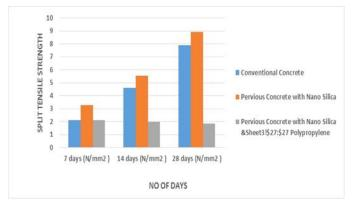
Figure 11 Results for Split Tensile Strength
