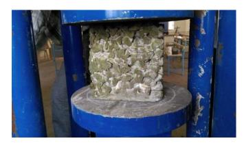
Figure 6 Compression Test
