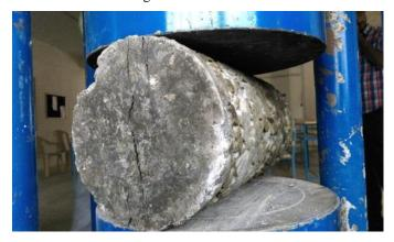
Figure 8 Split Tensile Test
