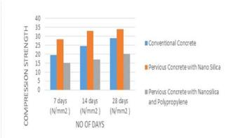
Figure 11 Results for Compressive test
