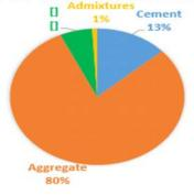
Figure 2 Pervious Concrete Ingredients
